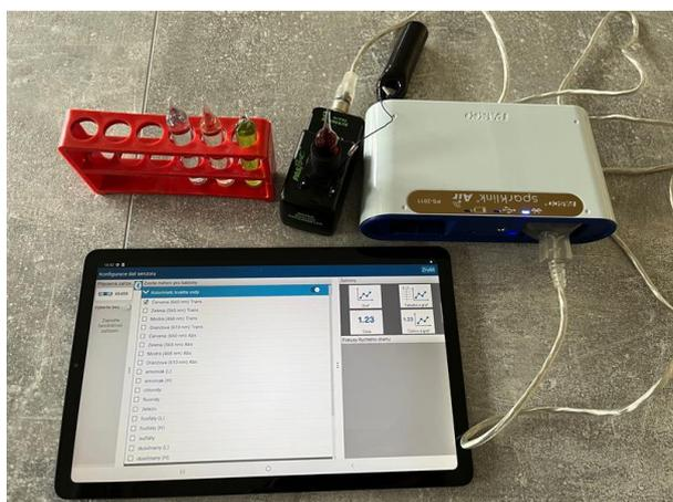
**Sparklink** – for measuring you'll need again chemicalls and then tablet. When we have chnchemicals, we connect Sparklink to the tablet (as you can see on photo) and add the chemicalls in the black device. Then we cover the chemicalls with black top (because it also, as the Colorimetr, uses light to measure, but kinda different) and find on tablet value, that we are measuring. Then we start measure.
