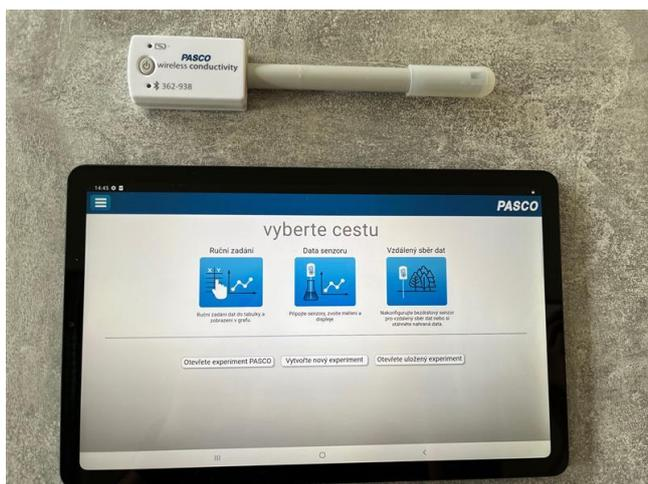
**PASCO wireless Conductivity** – we measure with this conductivity of water. We do the same, as we did oxygen.
